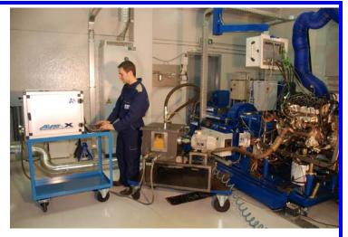
To cover a wide range of applications, the aeration measurement can be performed either directly in the output line of the generator, or at a selected point in the mechanical system under test. Whatever the sampling point, the generator will increase automatically the aeration level in the supply line until a pre-defined value is reached at the sampling point.
