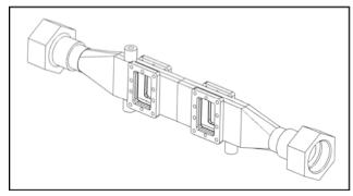
The core of Air-X is a compact measuring chamber with 2 windows: one is used for the X-ray transmission measurement, the other for the visualisation of the oil flow via a video system.
