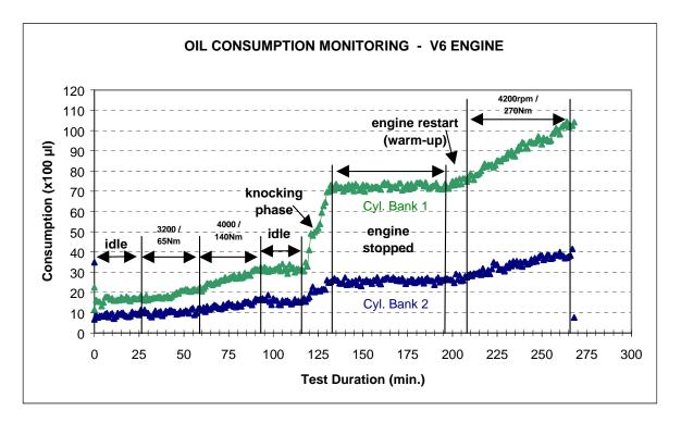
As expected, higher speeds and loads are associated to higher lubricant consumption. It also appears clearly that consumption of cylinder bank 1 is significantly higher than bank 2. Between t=110 and t=130 min., the sudden oil consumption increase was due to particular conditions that induced engine knocking.
